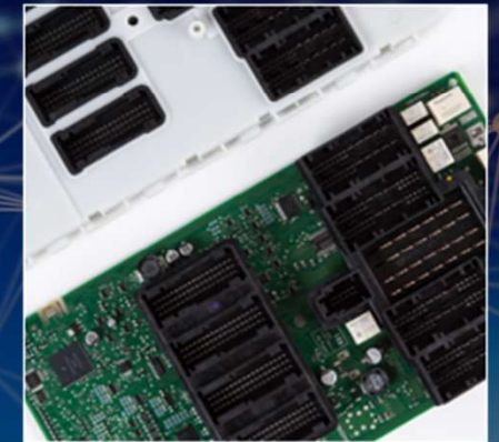
Zone Control Module (Electronics)
